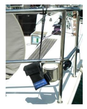
2. Wrap the Velcro straps around horizontal and vertical rails as shown below.
