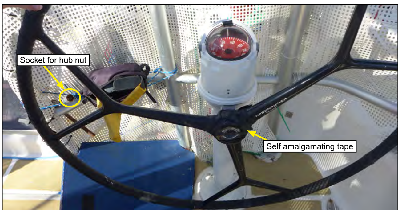
Figure 37: Starboard wheel temporary repair with socket spanner accessible to tighten hub nut
