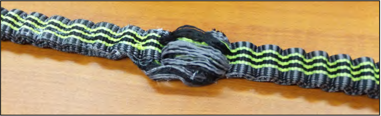
Figure 29: Frayed elasticated section of long tether
