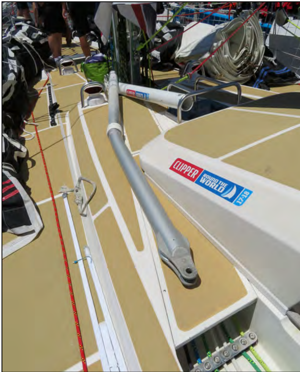
Figure 4: Buckled vang strut
