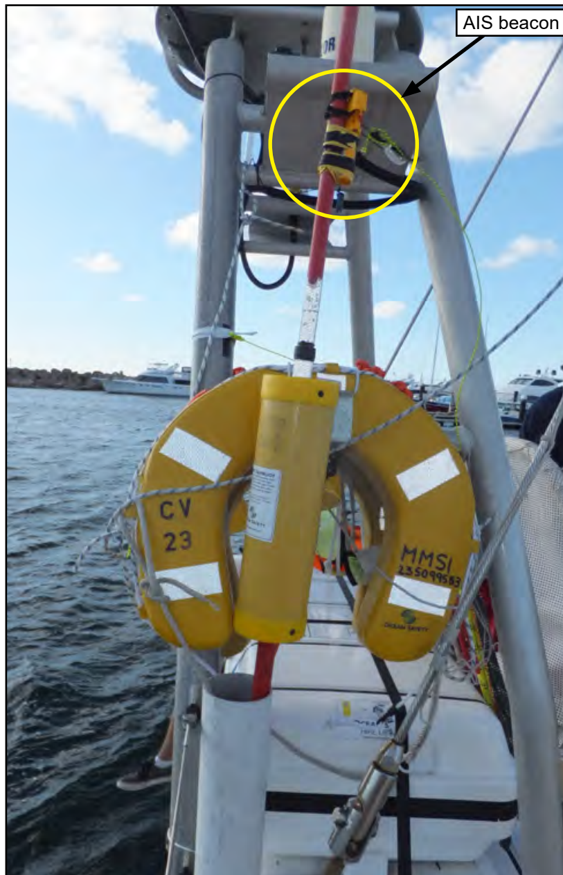
Figure 35: Dan buoy and horseshoe life-ring showing AIS beacon
