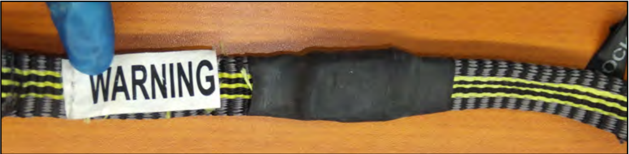
Figure 30: Safety tether overload indicator
