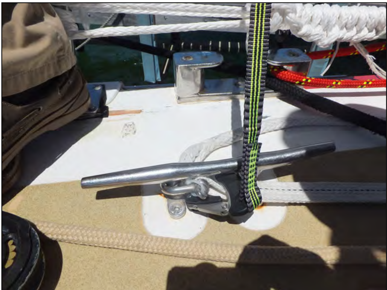
Figure 32: Tether hook caught under cleat attached to primary jackstay
