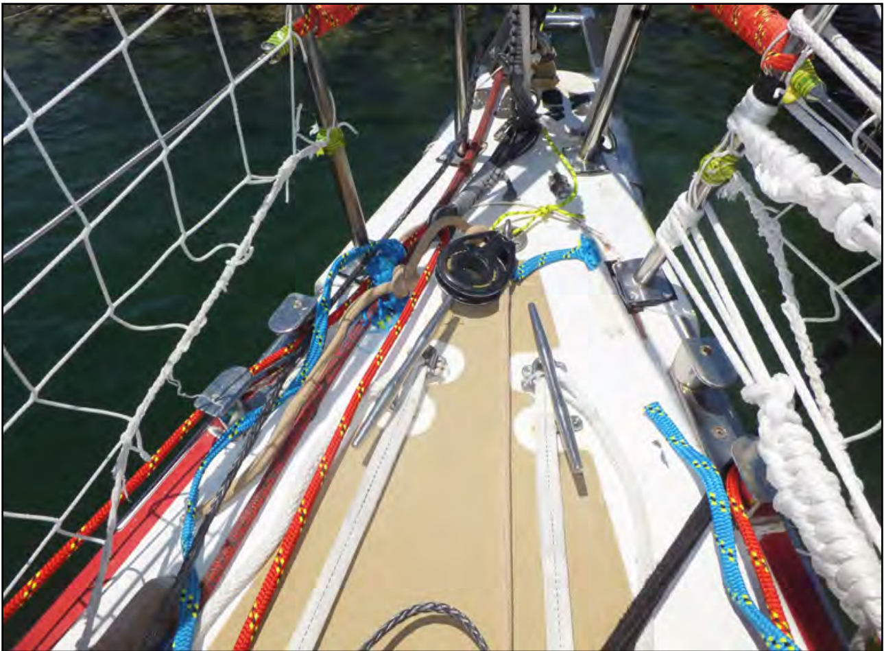
Figure 20: Attachment of jackstays to bow cleats
