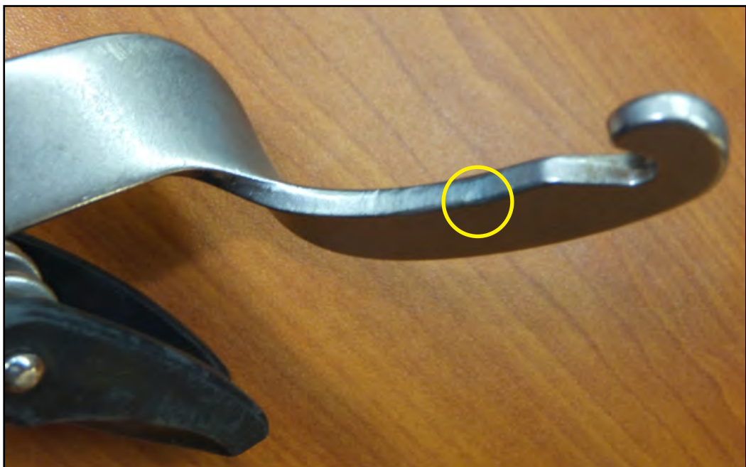
Figure 27: Distorted tether hook small indentation (circled)
