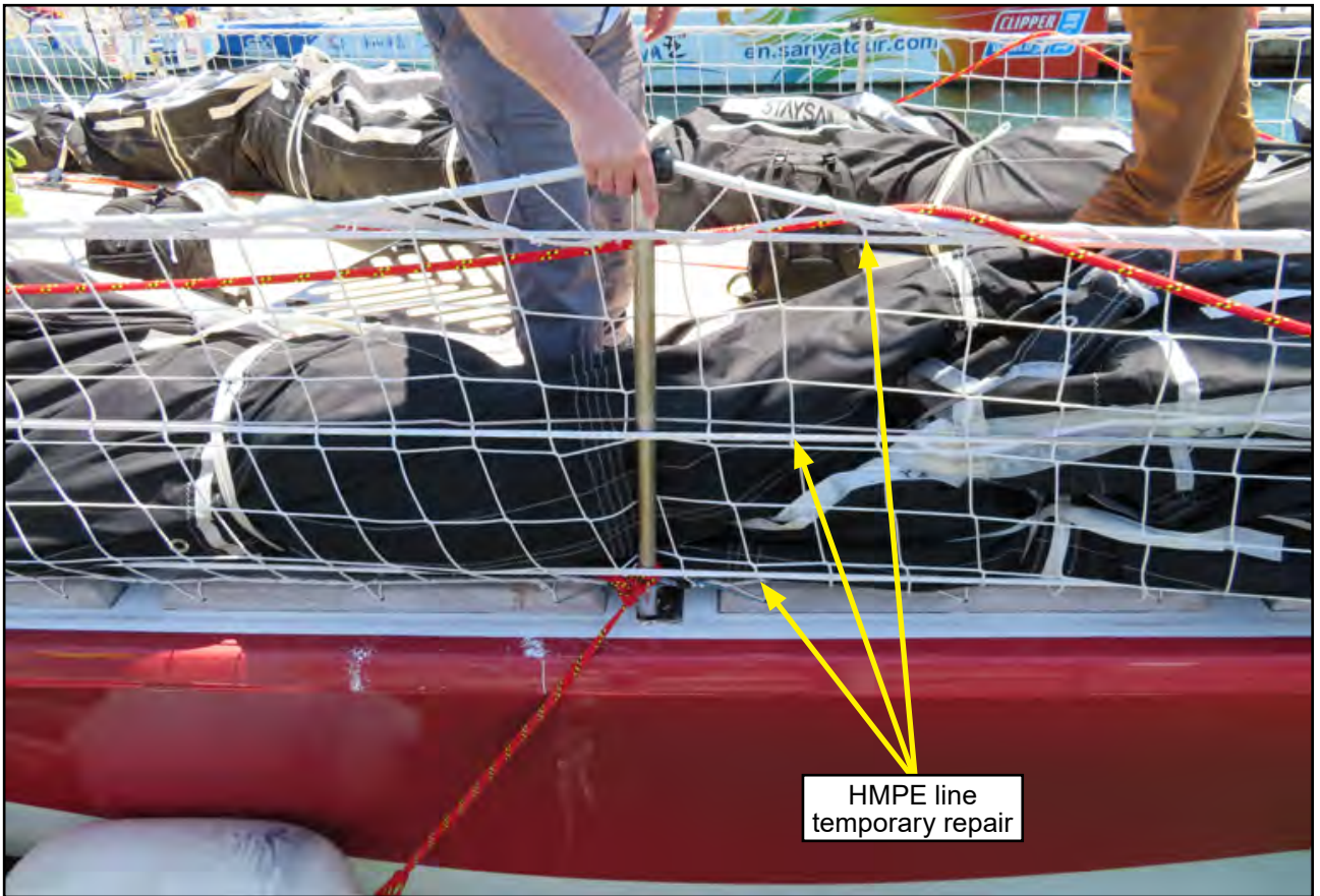
Figure 2: HMPE line temporary repair of guardrail
