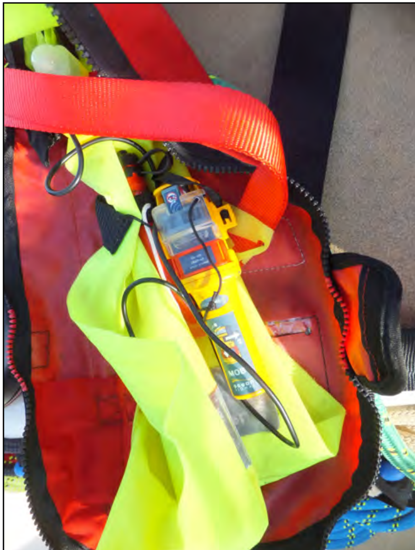
Figure 34: Ocean signal MOB1 AIS beacon fitted to lifejacket
