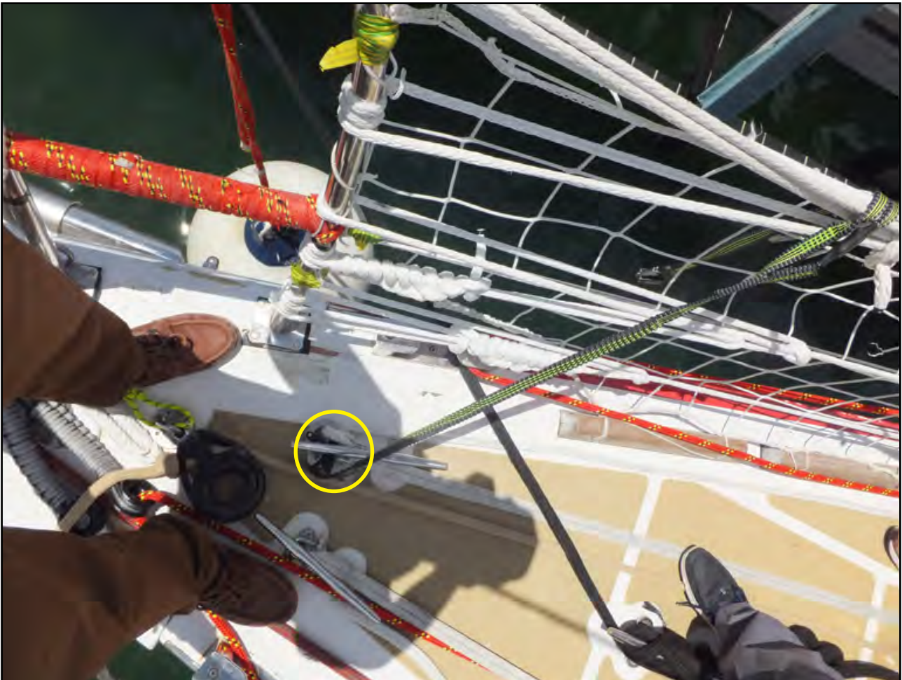
Figure 9: Reconstruction showing tether hook caught under bow cleat, as observed by bowman
