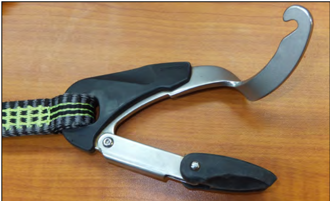
Figure 26: Distorted tether hook
