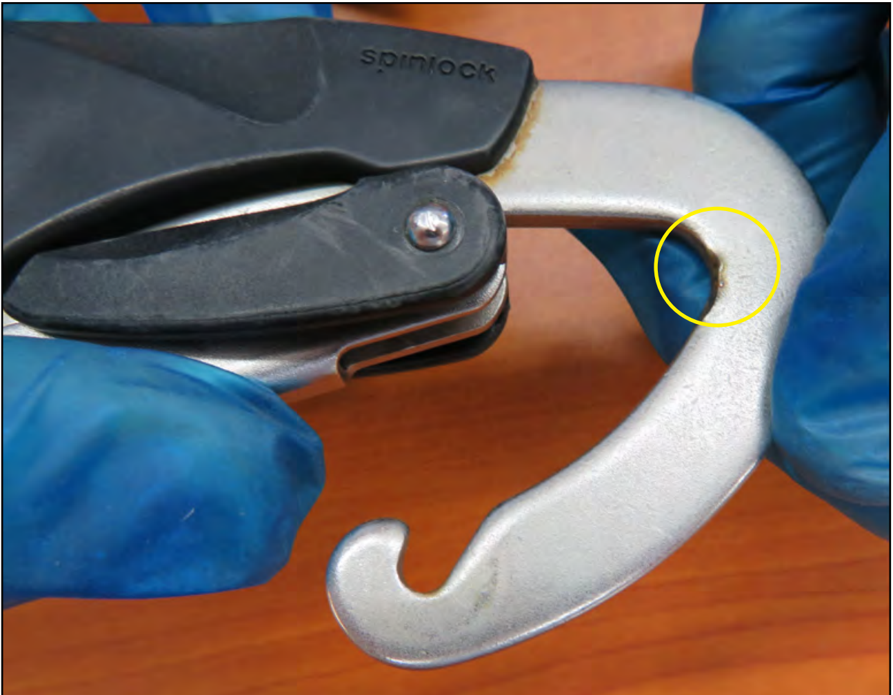
Figure 28: Tether hook secured to harness notching
