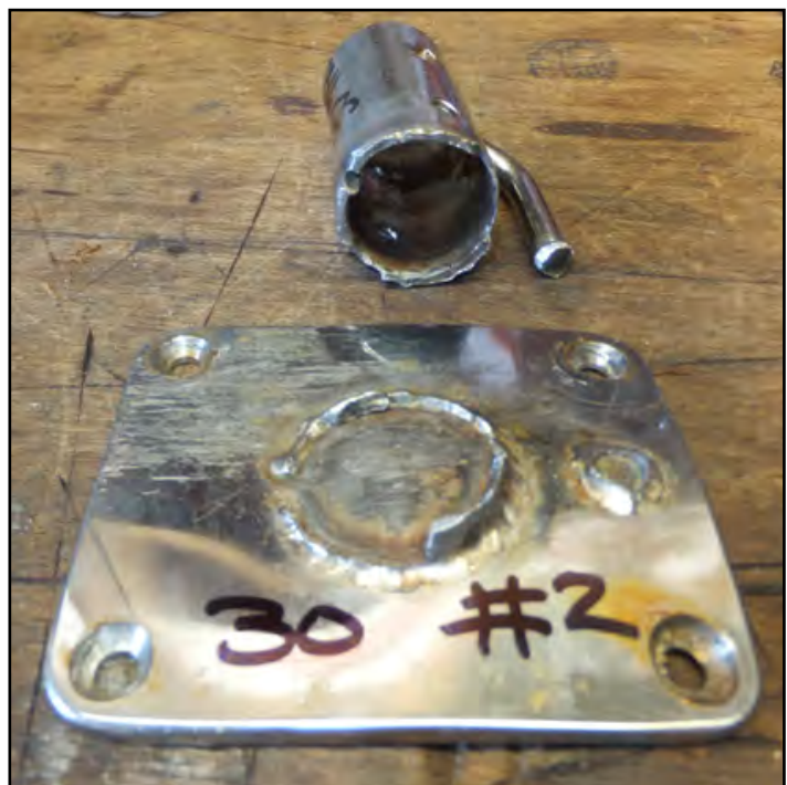
Figure 17: Fractured stanchion base
