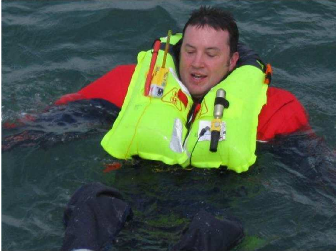
Figure 5 - An example of an AIS SART the Kannad SRS R10 fitted to the right hand yoke, aerial deployed
