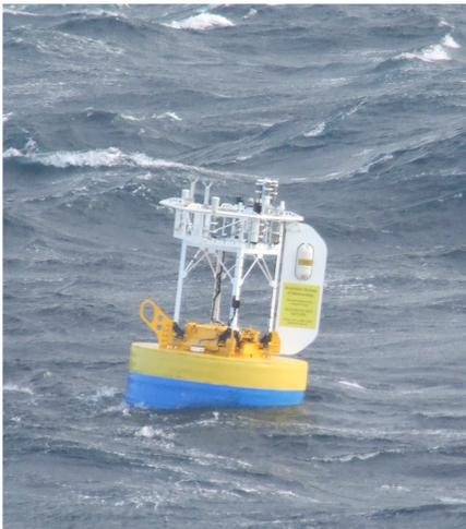
Keeping a lonely vigil on the weather 600 kilometres southwest of Hobart in a depth of four and a half kilometres is a buoy that is a first for the Southern Ocean. The Southern Ocean Flux Station (SOFS) was deployed in March this year and has been transmitting data in real time back to the Bureau of Meteorology
